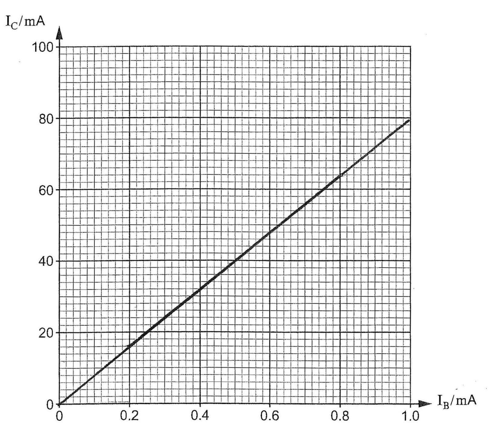
Determine the current gain  $(h_{FE})$  of the transistor.
