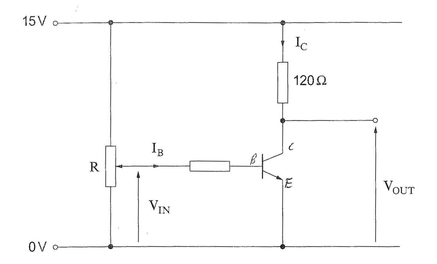
Potentiometer R is varied and readings of  $V_{\rm IN},\,V_{\rm OUT},\,I_{\rm B}$  and  $I_{\rm C}$  are taken.
