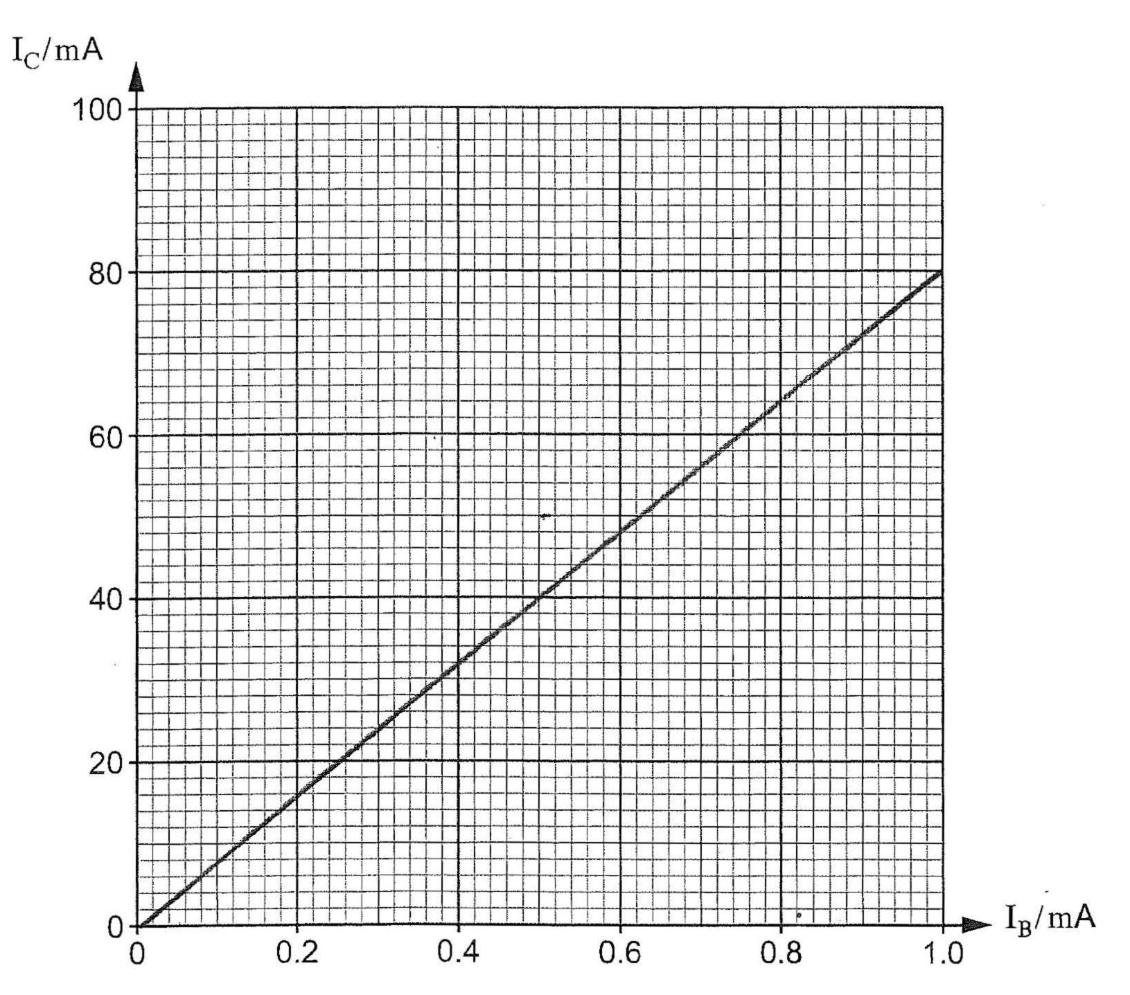
(ii) Determine the current gain  $(h_{\rm FE})$  of the transistor.
