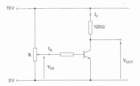
Potentiometer R is varied and readings of  $V_{IN},\,V_{OUT},\,I_B$  and  $I_C$  are taken.
