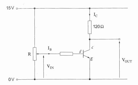
Potentiometer R is varied and readings of  $V_{\rm IN},\,V_{\rm OUT},\,I_B$  and  $I_C$  are taken.
